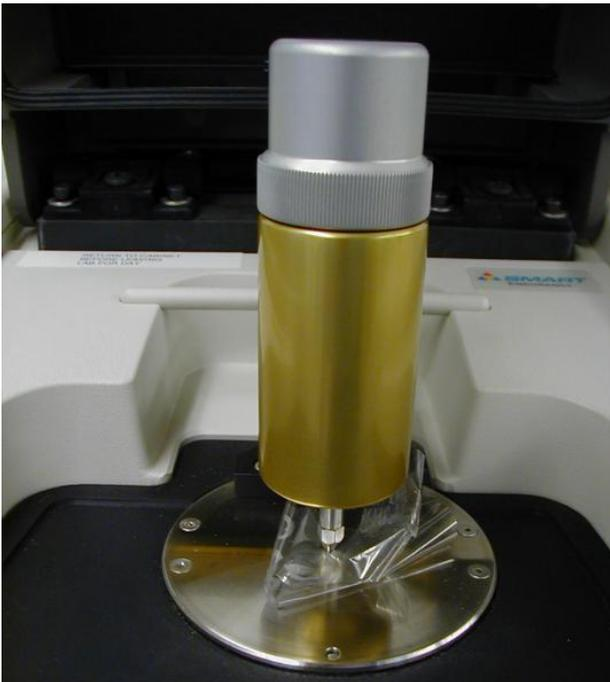
Anvil with plastic film sample pressed onto sample cell window.
